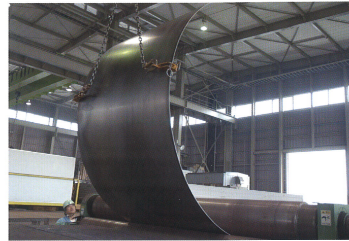
◀ Steel sheet bending process
