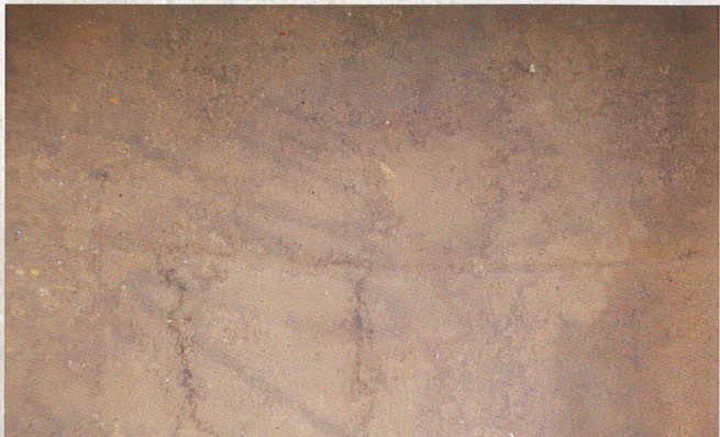
Corrosion due to water accumulation at the bottom of a tank after more than 40 years of use
